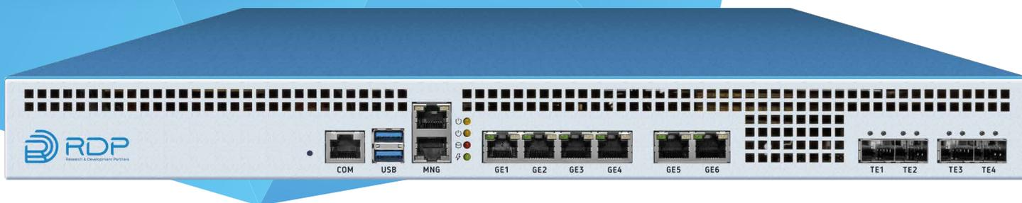
**EcoFilter** is an operator-grade product which assures URL filtering of entire provider's traffic on the wire speed and blocks 100% of prohibited resources according to the Roskomnadzor's register (RKN), Ministry of Justice, and to the provider's lists.
